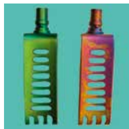
Fig. 4: The colour change usually occurs evenly. However, it may also appear patchy/multi-coloured.
